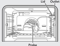
3. Flip up the lid of the outlet, located on the upper right side of the oven cavity. Insert the probe into the outlet and close the oven door. The probe temperature will display <----°> in the text window and the meat probe indicator will flash.
